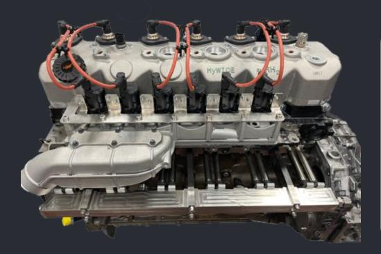
"Thanks to a mechatronic spacer mechanism, RH2 replaces diesel fuel with a double direct injection of hydrogen and water."
